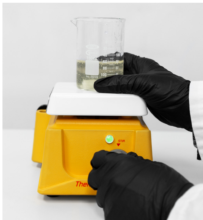
Figure 2: Dilution of NovaFilm™ Gel Base using a magnetic stirrer.
